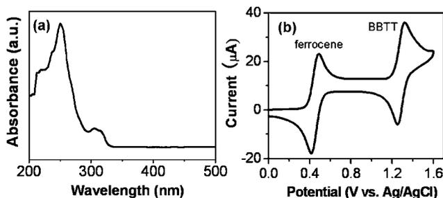
Fig. 1 (a) UV-vis absorption spectrum of BBTT in CH<sub>2</sub>Cl<sub>2</sub> ( $\sim 10^{-5}$  M), (b) cyclic voltammogram curve of BBTT using Ag/AgCl as reference electrode and ferrocene as internal standard.
