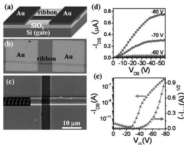
**Fig. 5** (a) Schematic diagram and (b, c) optical and SEM images of example OFETs based on individual BBTT single crystal ribbons, (d, e) typical output and transfer characteristics of the devices (here channel length  $L = 4.9 \mu\text{m}$ , channel width  $W = 5.4 \mu\text{m}$ ).
