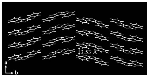
Fig. 2 Crystal packing of BBTT in the *a*-*b* plane with molecular packing distance along the *a* direction at 3.53 Å.
