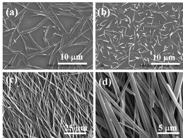
Fig. 3 (a, b) SEM images of vacuum deposited films of BBTT on SiO<sub>2</sub> and OTS modified SiO<sub>2</sub> substrates. (c, d) SEM images of micro- and nanoribbons of BBTT self-assembled by drop casting from saturated toluene solution.
