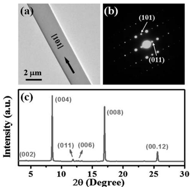
**Fig. 4** (a) TEM image and (b) corresponding SAED pattern of an individual ribbon. (c) XRD pattern of the self-assembled single crystal-line ribbons of BBTT on OTS modified SiO<sub>2</sub> substrates.
