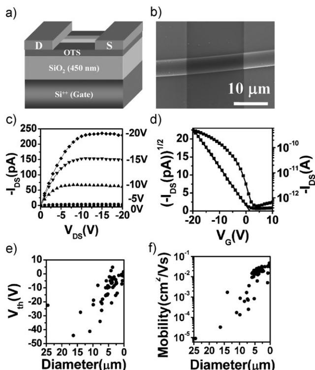
**Figure 5.** a) Schematic diagram and b) SEM images of the devices with an individual ribbon, c) output and d) transfer characteristics (channel length,  $L = 17.9 \mu\text{m}$ , channel width,  $W = 190 \text{ nm}$ ) of the devices, and e) mobility and f) threshold voltage distribution of 50 devices as a function of crystal size.
