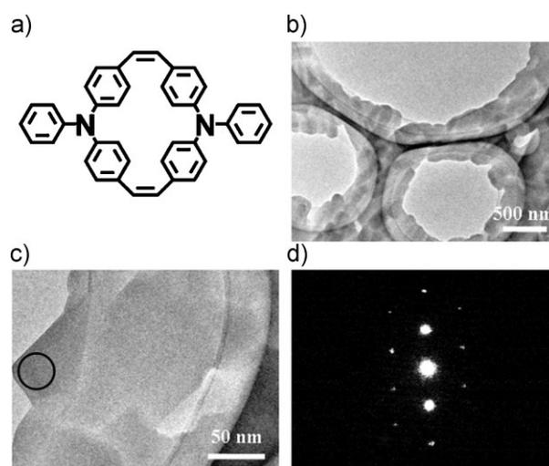
**Figure 1.** a) Chemical structure of compound 1. b) TEM image of the deposited film over a large area on a copper grid. c) TEM image of an enlarged area, and d) the corresponding SAED pattern of the selected area (the circled area in c).
