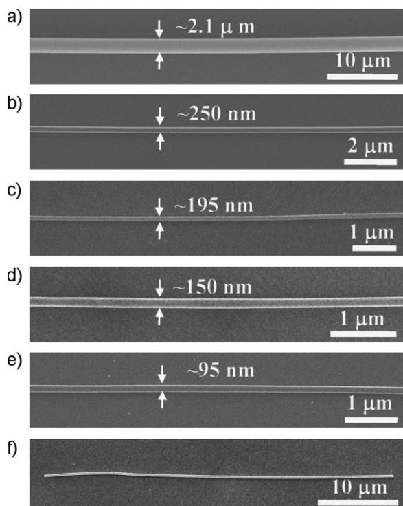
**Figure 4.** In situ patterned ribbons of compound **1** with different size on OTS-modified SiO<sub>2</sub>: a) 2.1 μm, b) 250 nm, c) 195 nm, d) 150 nm, e) 95 nm, and f) an individual ribbon several tens of micrometers long.
