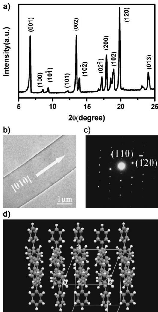
**Figure 3.** a) Powder diffraction pattern of the ribbons. The peaks were indexed with lattice constants of the bulk crystal. b) TEM images of an individual ribbon and c) the corresponding SAED pattern, indicating that the ribbons grow along the  $[010]$  direction. d) Molecular arrangement in the ribbon.
