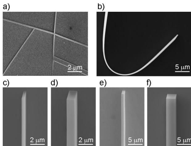
**Figure 2.** a) Nanometer- and micrometer-sized ribbons of compound 1 produced by the physical vapor transport technique. b) An individual bent ribbon of several tens of micrometers in length. Ribbons with different diameters: c)  $\sim 250$  nm, d)  $\sim 500$  nm, e)  $1 \mu\text{m}$ , and f)  $4 \mu\text{m}$ .
